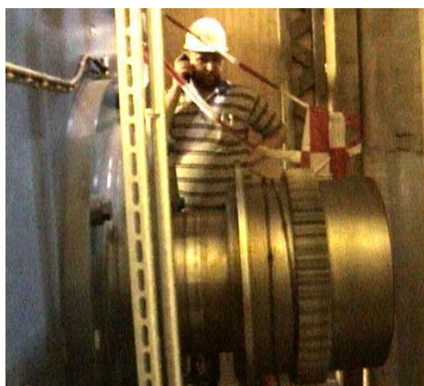
Fig. 6: View on the uncoupled motor shaft.
